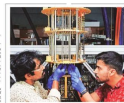
TIFR scientists wire up a dilution refrigerator used to cool superconducting qubits to -273.14°C for building a small-scale quantum processor. (TIFR)
