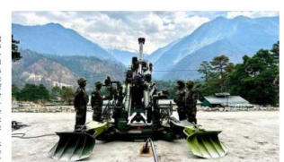
Long range: The M77 ultra light howitzer is a 125-mm, 30-calibre towed artillery gun, 20000 100
